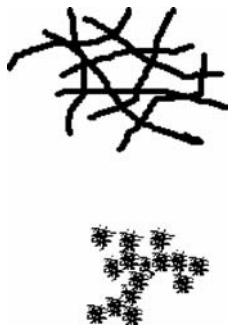
Figure 5. The structure of typical silica colloids obtained via polycondensation in acidic (upper image) and basic media (below) respectively.
