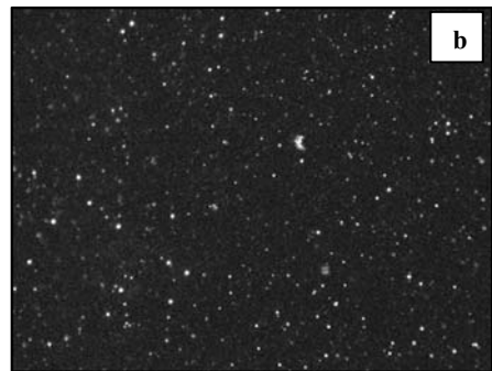
Figure 7. Micrographs of the colloidal nanosized silica (aerosil A-90): (a) – with NaOH, (b) – without stabilizer.
