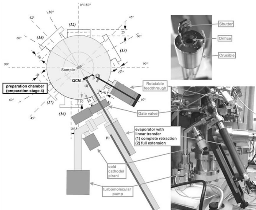
**Fig. 2.4** Sketch and photo of the IL evaporator setup. With this setup the evaporator can be detached from the chamber, for refilling or change of IL. Furthermore, the IL can be introduced to the chamber after bake-out, which is a crucial point as the IL evaporation temperature lies in the range of the bake-out temperature
