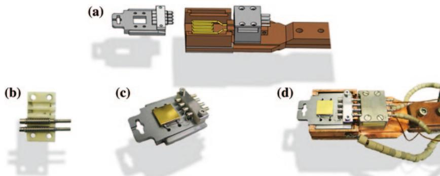
**Fig. 2.5** Sketch (a) and pictures (b–d) of the sample holder system. The pins on the sample holder and the spring-loaded counter-notches (b) fitted to the manipulator head are made of type K thermocouple material. Once inserted into the manipulator, the springs push the sample holder back into its locked position (c), which guarantees both good electrical contact as well as firm and accurate mechanical interlock
