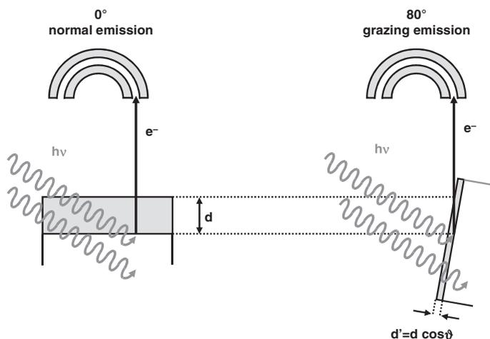
**Scheme 2.2** Illustration of the ARXPS setup. The information depth  $d'$  results from the cosine of the tilt angle with respect to the surface normal, therefore at 80° the surface sensitivity of XPS can be enhanced by a factor of six
