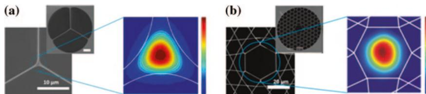
**Fig. 5.1** Overview over two different PCF cross sections; **a** “Mercedes” fibre, where the light is guided in the solid core in the middle of the fibre, and **b** “Kagome” fibre, which is a hollow core band gap fibre, in which the light is guided in the hollow cavity of the fibre. For details, see Ref. [5]
