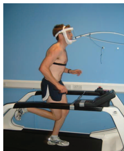
Athlete completing time trial while being exposed to ozone (100 parts per billion) via a face mask system
