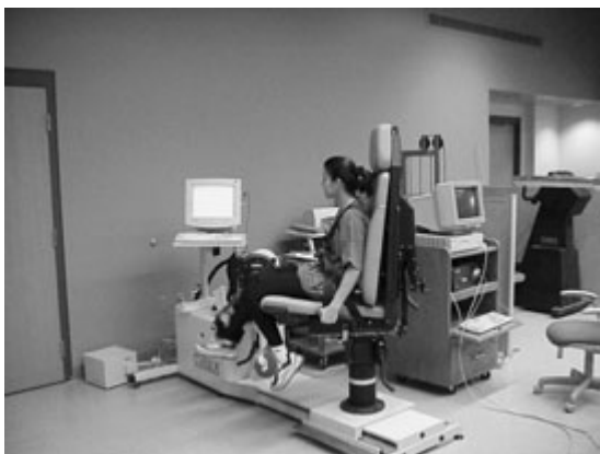
Fig. 4.6 Isokinetic dynamometer set-up for assessment of knee extensor and flexor muscle performance.
