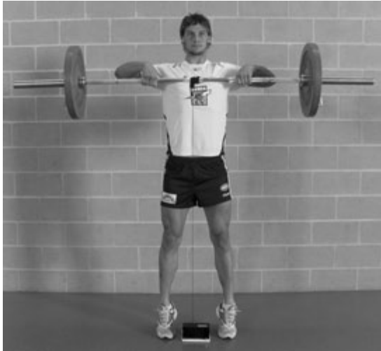
Fig. 4.5 Displacement transducer for measurement of linear movement. Velocity, acceleration, force, and power output can be estimated using the inverse dynamics approach.
