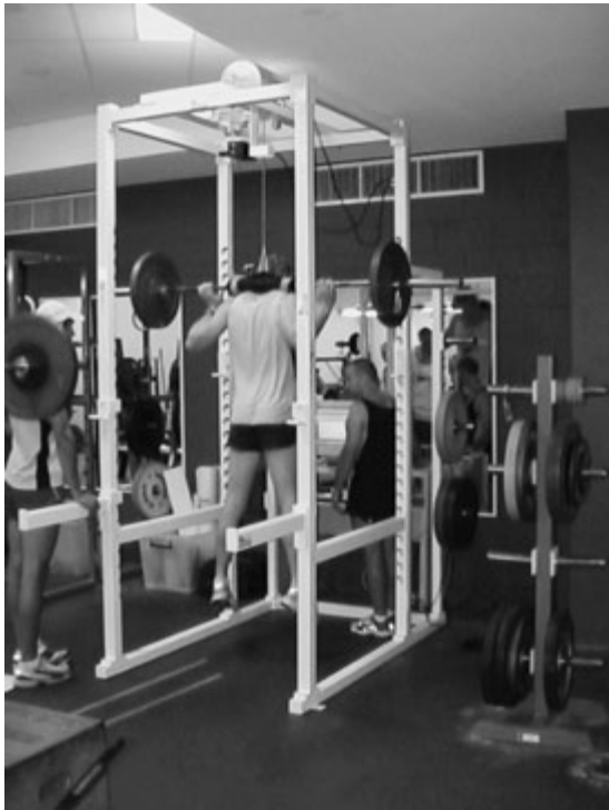
Fig. 4.11 Electromagnetic brake device used to reduce impact forces during ballistic resistance training. The system can also be used to perform eccentric strength testing using loads in excess of the concentric 1 RM.
