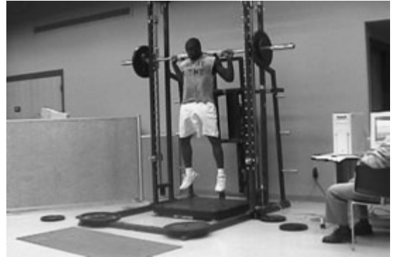
Fig. 4.7 Measurement of power output in a squat jump for determination of optimal load for power production. Ground reaction force measured by force platform is used to calculate velocity and subsequently power output.
