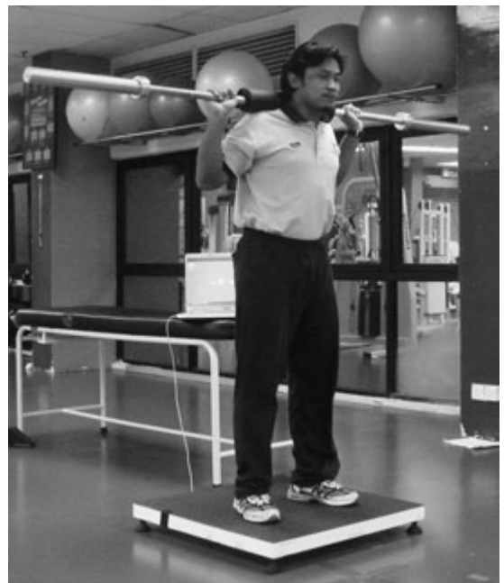
Fig. 4.3 Force platform for measurement of strength and power qualities.
