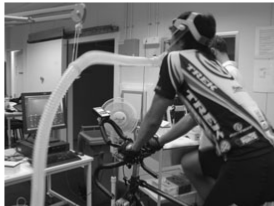
Fig. 4.16 Subject breathing into a metabolic cart while performing a progressive exercise test on a cycle ergometer for the determination of maximal oxygen uptake, anaerobic threshold, and cycling economy.
