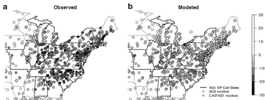
Fig. 71.1 2005–2002 difference in the average of the top ten summer MDA8 ozone values (ppb) at AQIS sites (circles) and CASTNET sites (diamonds)
