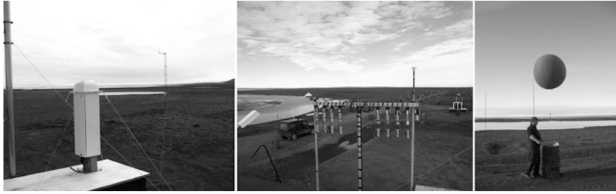
Fig. 86.2 Ceilometer and the 10 m mast for flux measurements ( left ), air quality measurements ( middle ) and releasing radio sonde, ( right panel )
