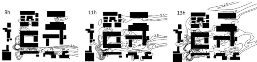
Fig. 57.2 Representation of hourly averaged PM10 concentration isolines ( \mu\text{g.m}^{-3} ) in a 1.5 m high horizontal plane. Buildings are shown as black rectangles and tree blocks were omitted for simplification
