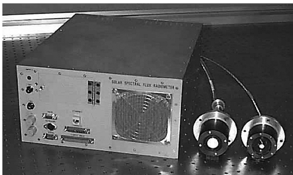
Fig. 6.1. Solar Spectral Flux Radiometer (SSFR) with zenith and nadir light collectors.
