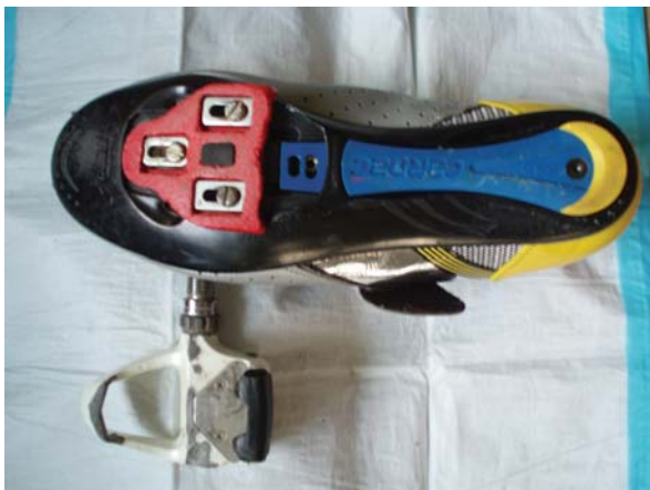
Fig. 18.1 Clipless pedal and cleat on outsole of shoe for road cycling
