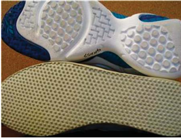
Fig. 19.3 Special “nub” outsoles on tennis shoes designed to increase traction on grass court surface
