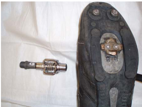
Fig. 18.2 Clipless pedal and cleat on outsole of shoe for mountain biking
