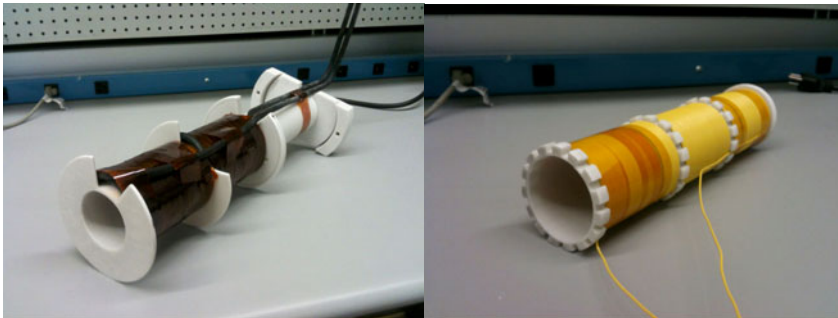
Fig. 3. Mouse transmit and receive coils. [LEFT] High power transmit coil wound with hollow core magnet wire. [RIGHT] receive coil wound with insulated wire.
