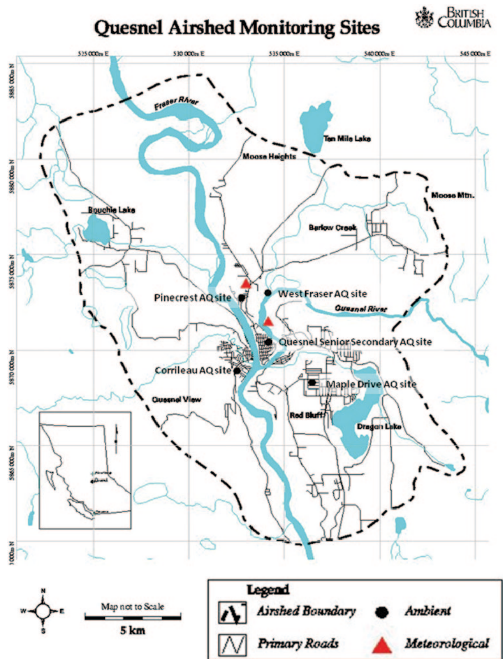
Fig. 17.3 Quesnel airshed map showing air pollutant and meteorological monitoring sites. (Quesnel Air Quality Roundtable 2004, Reproduced with permission from the BC Ministry of Environment)
