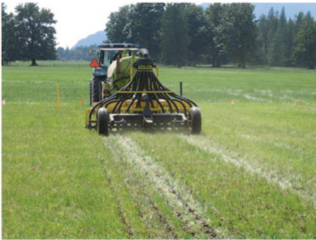
Fig. 11.11 A new low emission applicator for dairy slurry in the Lower Fraser Valley
