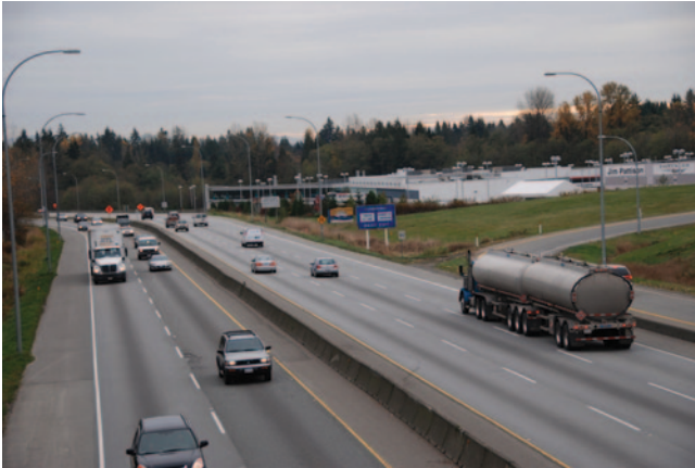
Fig. 5.7 Although not visible, these automobiles and trucks are emitting pollutants. Such roadway emissions are treated as a line source
