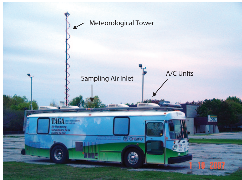
Fig. 1.3 Ontario Ministry of Environment TAGA Mobile Monitoring Unit (with permission from the Ontario Ministry of Environment)
