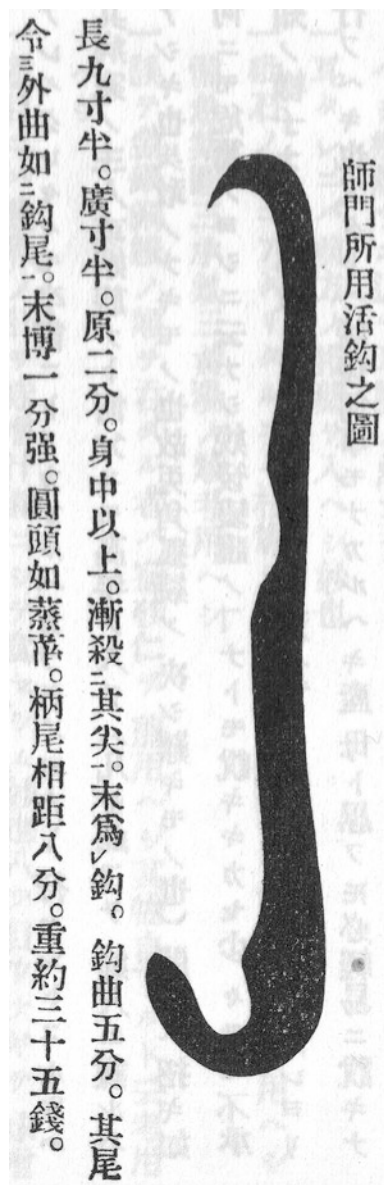
Fig. 3.11 An illustration of a hook used by Kagawa Gen'etsu, presented in Oku Ressai's obstetrics manual, Kaisei kōbō hikketsu . The size and weight of the hook are specified: length, nine-and-a-half sun ; and weight, 35 sen . The sizes of particular parts of the hook are meticulously described in the attached caption (1 sun = 3.03 centimeters = 1.193 inch; 10 bu = 1 sun ; 1 sen = 3.75 gram = 0.13 ounce). From Fujikawa et al. (1971: 764)
