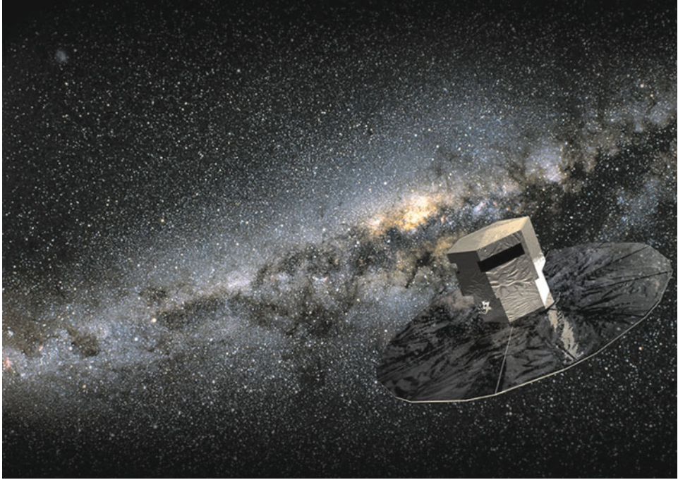
Figure 8.6 An artist's impression of the Gaia spacecraft against the background stars of the Milky Way. Gaia will conduct a census of a thousand million stars in our Galaxy, monitoring each of its target stars about 70 times over a five-year period, precisely charting their positions, distances, movements, and changes in brightness (ESA, illustration by Medialab).
