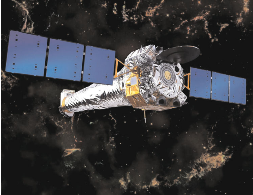
Figure 8.9 An artist's impression of NASA's Chandra X-ray Observatory, which was launched and deployed by Space Shuttle Columbia on 23 July 1999. Chandra is designed to observe X-rays emanating from very high-energy regions of the universe. The observatory has three major parts: the X-ray telescope, whose mirrors focus X-rays from celestial objects; the science instruments which record the X-rays so that X-ray images can be produced and analyzed; and the spacecraft, which provides the environment necessary for the telescope and the instruments to work. Chandra's unusual orbit was achieved after deployment by a built-in propulsion system which boosted the observatory to a high Earth orbit. This elliptical orbit takes the spacecraft more than a third of the way to the Moon before returning to its closest approach to the Earth of 16,000 kilometers. The time to complete an orbit is 64 hours and 18 minutes. The spacecraft spends 85 percent of its orbit above the belts of charged particles that surround the Earth. Uninterrupted observations as long as 55 hours are possible and the overall percentage of useful observing time is much greater than for the low Earth orbit of a few hundred kilometers used by most satellites (NASA Marshall Space Flight Center and the Chandra X-ray Center of the Smithsonian Astrophysical Observatory).
