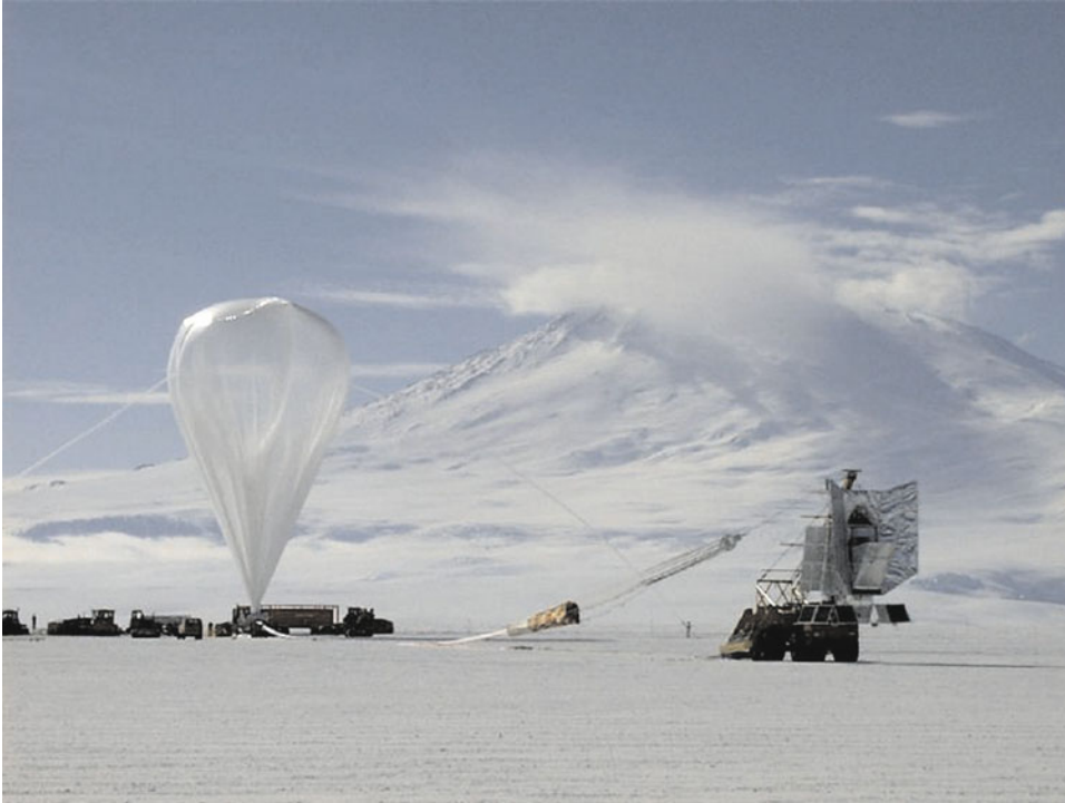
Figure 8.11 NASA/NSBF personnel inflate the one million \text{m}^3 balloon which will carry the BOOMERANG telescope on its 10-day trip around the Antarctic continent. In order to make its exquisitely sensitive measurements, BOOMERANG is lifted above 99 percent of the atmosphere to an altitude of 35 kilometers (120,000 ft.). The continuous sunlight and stable air currents over Antarctica enable 10 to 20 day long stratospheric balloon flights. This launch was preceded by two months of assembly at McMurdo research station, and half a decade of development and construction by a international team of researchers (NASA/NSBF).
