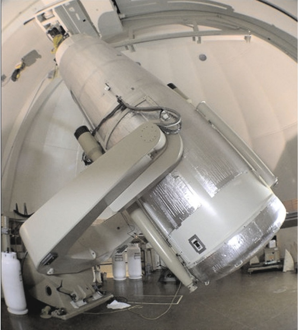
Figure 8.2 The 48-inch (1.22-meter) aperture Schmidt camera (the Samuel Oschin telescope), at the Mount Palomar Observatory in the USA. It was used for the first Palomar Observatory Sky Survey (POSS), which mapped the northern hemisphere of the sky during the 1950s (Palomar Observatory).
