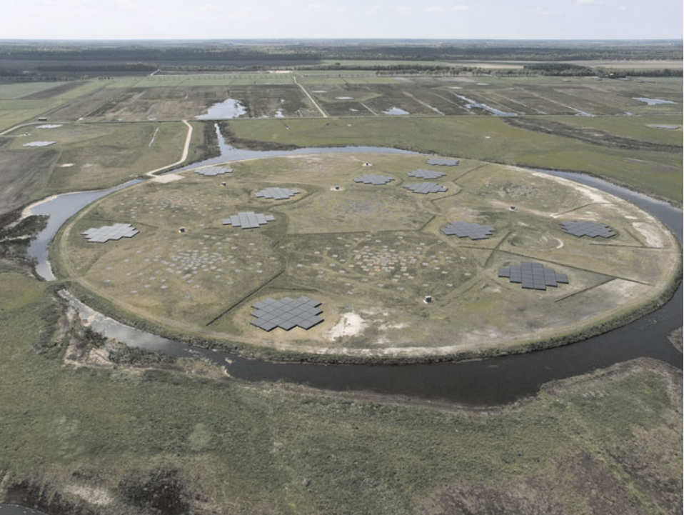
Figure 8.14 A view of the main core of the Low Frequency Array (LOFAR), located in the north-east of the Netherlands. LOFAR is a radio interferometer which observes the universe at low radio frequencies, close to the FM radio band, from 90 to 200 MHz. LOFAR is novel in its design because it is the first telescope which can look at the entire sky at the same time, unlike other telescopes which you have to point. In order to look in any given direction in the sky one uses a supercomputer to obtain information from a given direction. In addition to the many LOFAR stations in the Netherlands, others are located in France, Germany and one in the UK. One of the key LOFAR projects is to hunt for a signal from the epoch where the universe became re-ionized, most likely due to stars or quasars in the early universe emitting photons which ionized the diffuse gas in the intergalactic medium.. LOFAR will be able to probe this epoch by looking at the redshifted transition of the hyperfine structure in neutral hydrogen. This transition has a rest frequency of 1.4GHz, so if reionization happened at a redshift of around z = 8 then a radio interferometer would be able to map it (Netherlands Institute for Radio Astronomy (ASTRON)).
