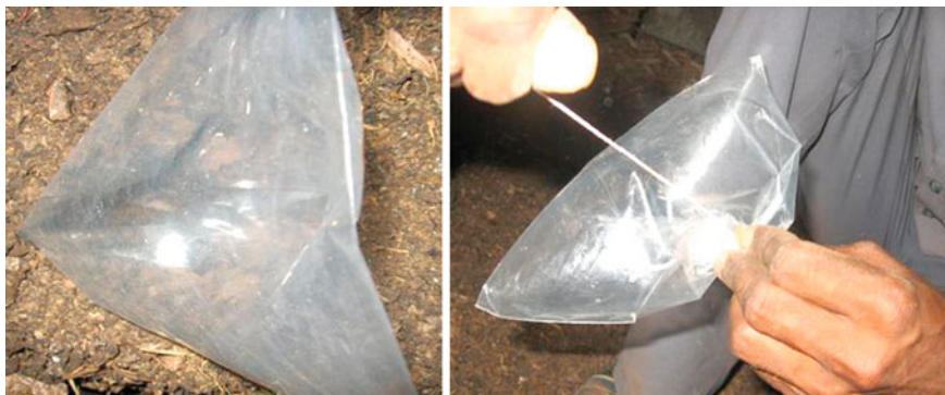
Fig. 6 Gas collection from compost plant
