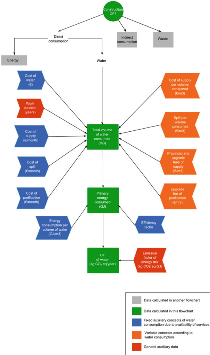
Fig. 7 Flowchart to determine the carbon footprint of water consumption. CF, carbon footprint
