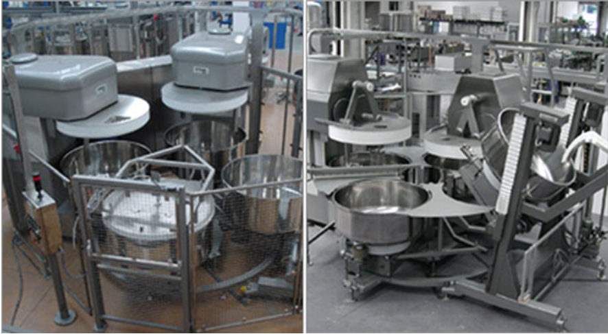
Fig. 3.6 Carousel system (Courtesy of Sancassiano S.p.A., Italy)
