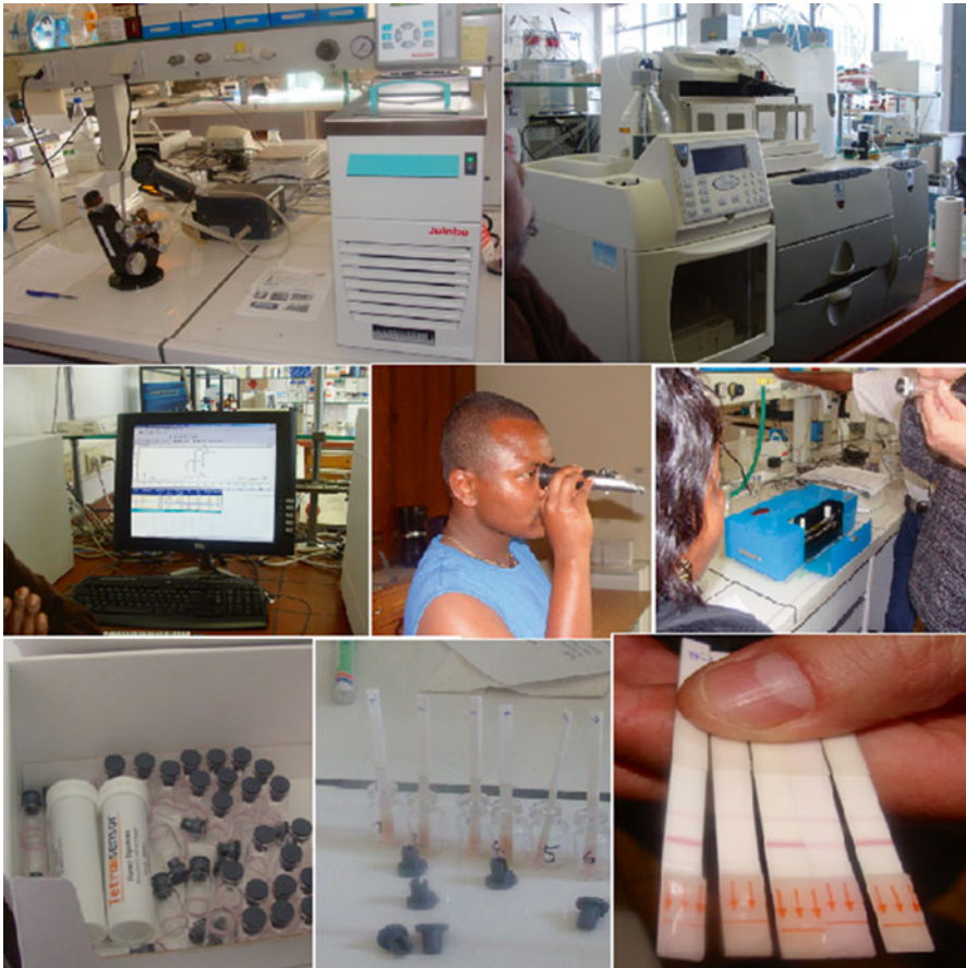
Fig. 22.1 Honey Quality lab at Institute for Agricultural and Fisheries Research (ILVO) Technology and Food Science Unit in Melle, Belgium. Top to Bottom (L–R): first row Equipment used for moisture and sugars in honey second row: A computer based interpretation on HMF, refractometer for determination of moisture content in honey, polarimeter used for determination of specific rotation third row: A Tetrasensor Honey kit for antibiotic residues (tetracyclines), performing this simple test, interpretation of results
