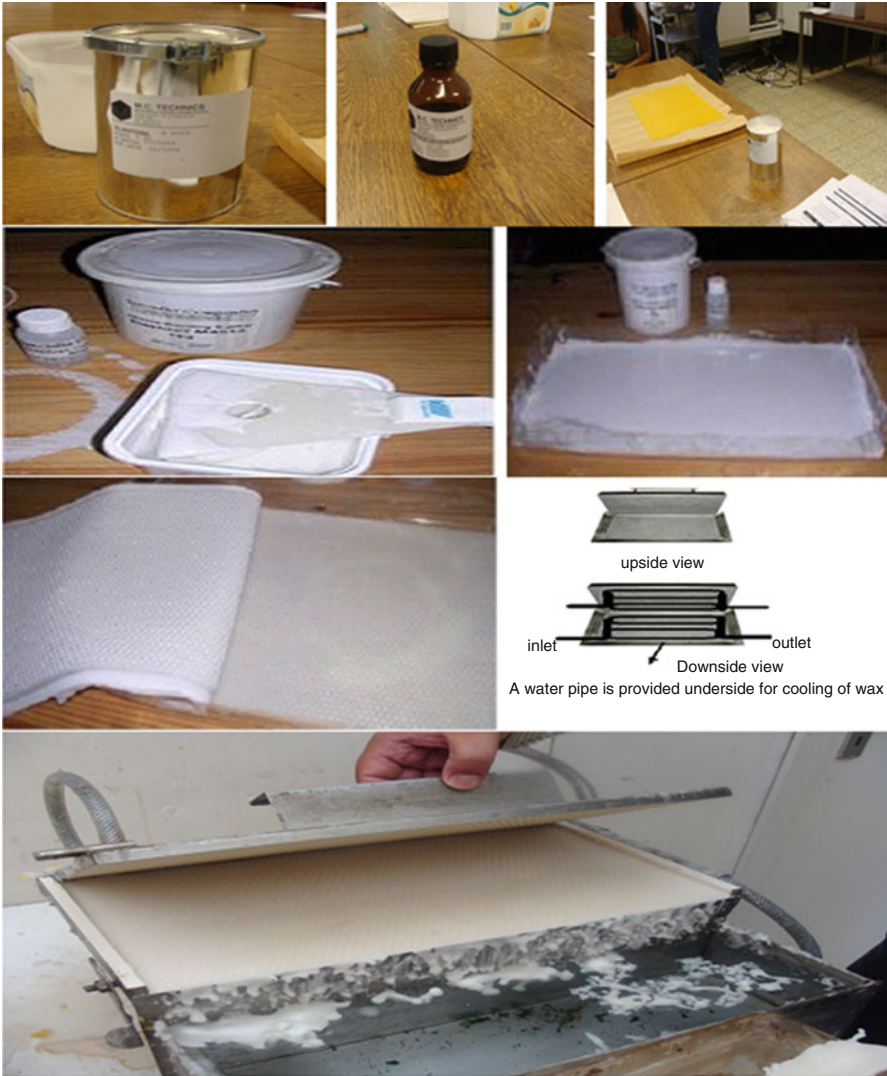
Fig. 19.3 Naturalizing cell size of worker foundation: making your own wax foundation machine for conserving bees
