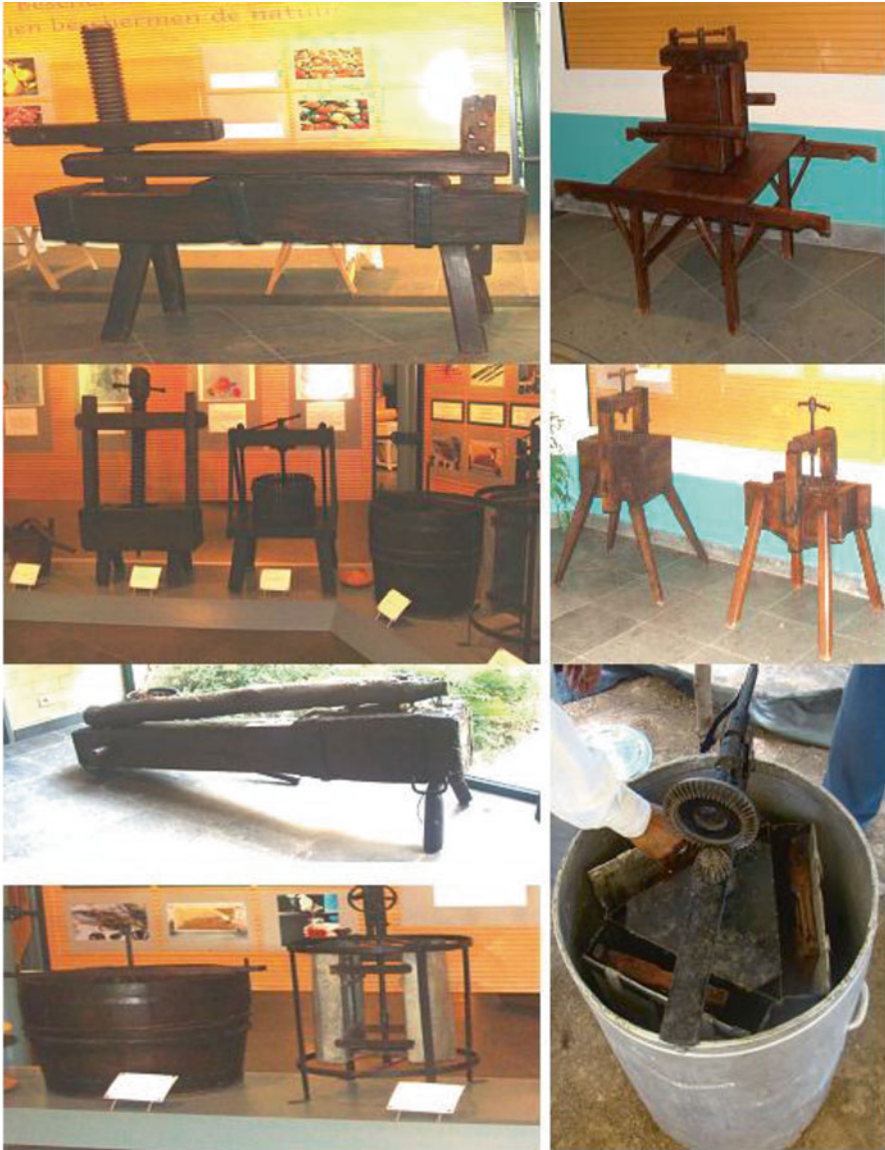
Fig. 1.4 Development of honey extractor: from traditional honey press to centrifugal extractors
