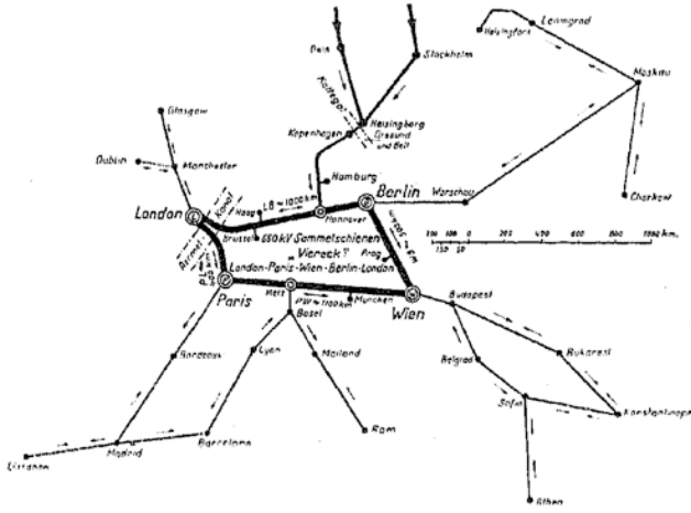
Figure 3.2d A European grid plan by Schönholzer. Source: Schönholzer 1930. Used by permission of the Schweizerische Technische Zeitschrift.
