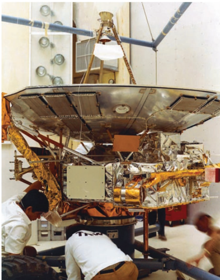
Figure 15.3 Photograph of the Pioneer F spacecraft at NASA's Kennedy Space Center, February 1972, with plaque attached to struts, shown at center of photograph. The plaque surface containing inscriptions of images and symbols that comprise the interstellar message is faced inwards towards the center-line of the dish antenna to avoid erosion during its journey through interstellar space.
