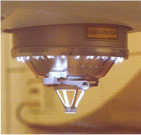
Figure 5-6 Intralase femtosecond laser with cone attached. (Reproduced with permission from Feder RS, Rapuano CJ. The LASIK Handbook: A Case-Based Approach . Philadelphia: Lippincott Williams & Wilkins; 2007:45, fig 2.7. Photograph courtesy of Robert Feder, MD.)
