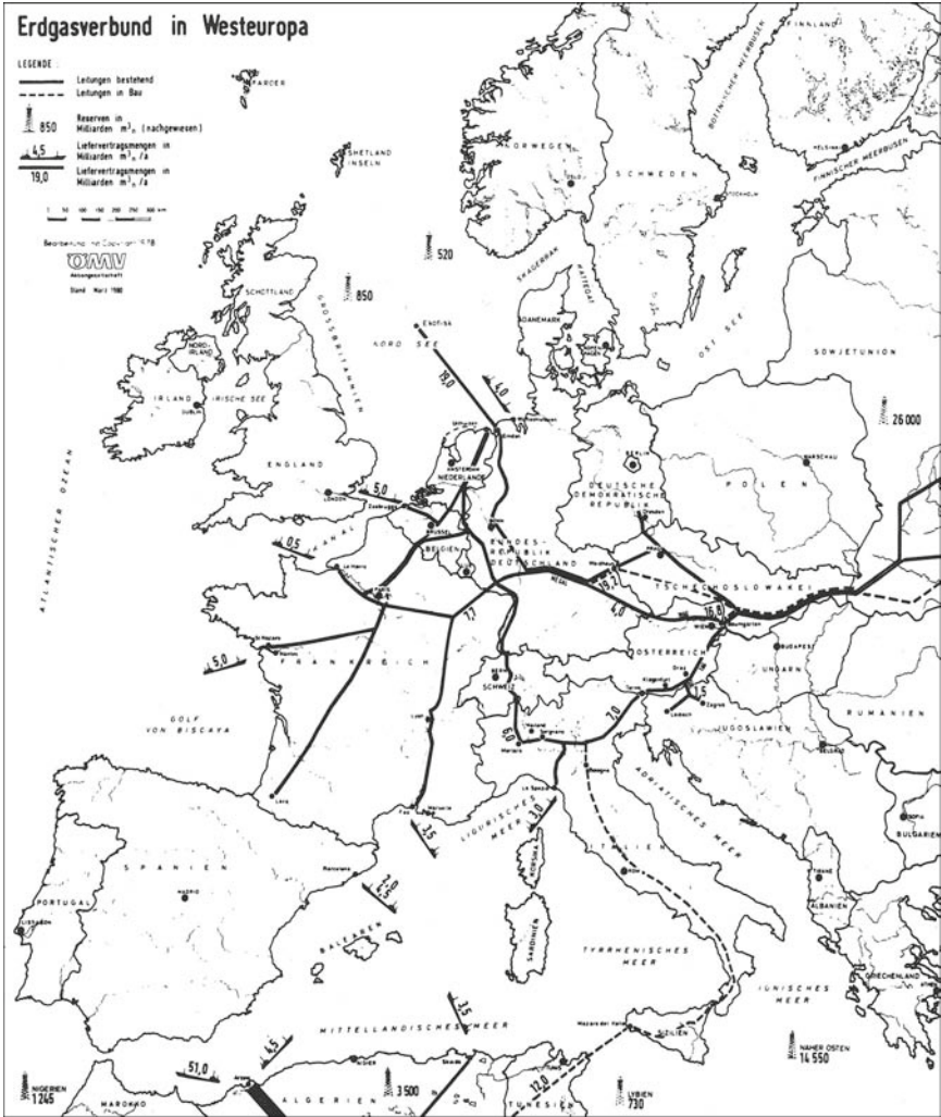
Figure 10.3 The integrated gas system of Western Europe as of 1980. This map from ÖMÖV makes visible the ways in which the export pipelines from the Soviet Union contributed to Western Europe’s internal integration.
