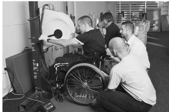
Figure 14.7 For a Wingate test, the athlete sits in his/her own braked daily use wheelchair held by two research team assistants. (Photo courtesy of Mariola Godlewska)
