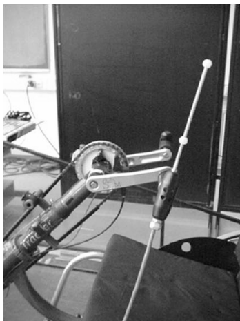
Figure 2.3 Instrumented handle bar with 6 degrees of freedom to measure forces and torques in 3D.
