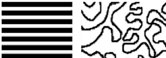
Fig. 1.14 Crystalline polymers: regular domains, amorphous polymers, coiled irregular domains
