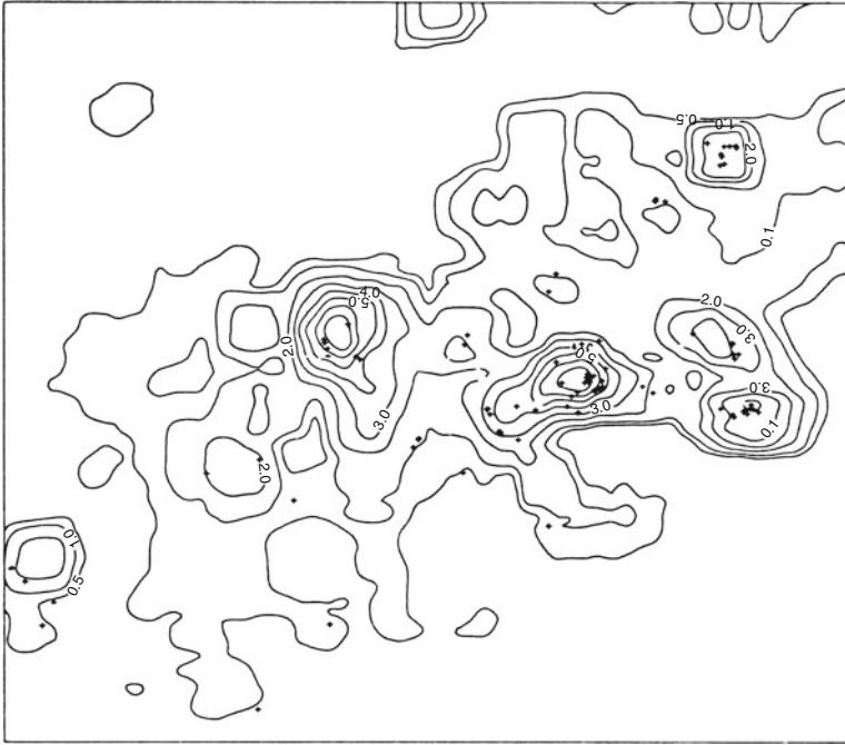
Fig. 5.21 Automatic contour map for occurrence of copper-zinc deposits; linear model applied to 38 lithological variables; contour value represents expected number of (10 km × 10 km) cells containing one or more Cu-Zn deposits per (40 km × 40 km) unit area; crosses represent known Cu-Zn deposits; see Fig. 5.20 for location (Source: Agterberg 1974, Fig. 3)
