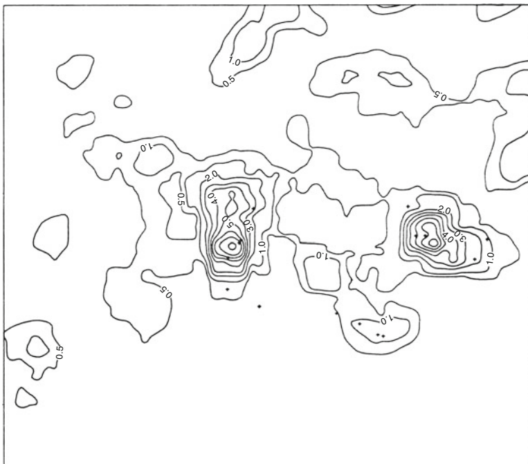
Fig. 5.22 Occurrences of nickel-copper deposits as predicted by linear model as in Fig. 5.21 (Source: Agterberg 1974, Fig. 4)
