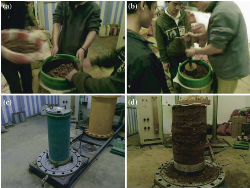
Fig. 7.11 Triaxial test. a fill, b compact, c test, d discharge.
