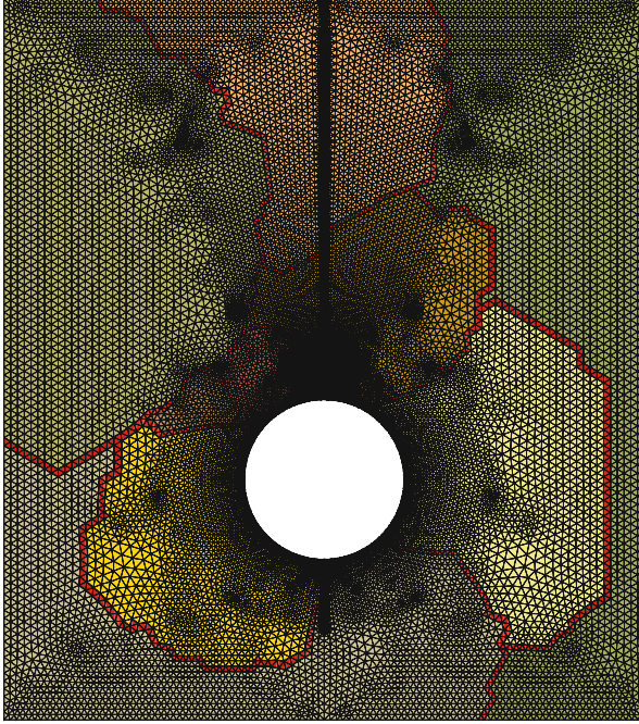
Fig. 8.15 Example of a partitioned 2D triangle mesh: Elements drawn in red indicate the border set partition \Omega^0
