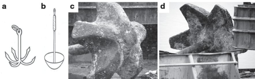
Fig. 1.2 Modern nautical anchors. a Grapnel anchor—pointed and flattened flukes. b Mushroom anchor for small boats—rounded bottom. c, d Large mushroom-type anchor on a US Navy barge, Ketchikan, Alaska
