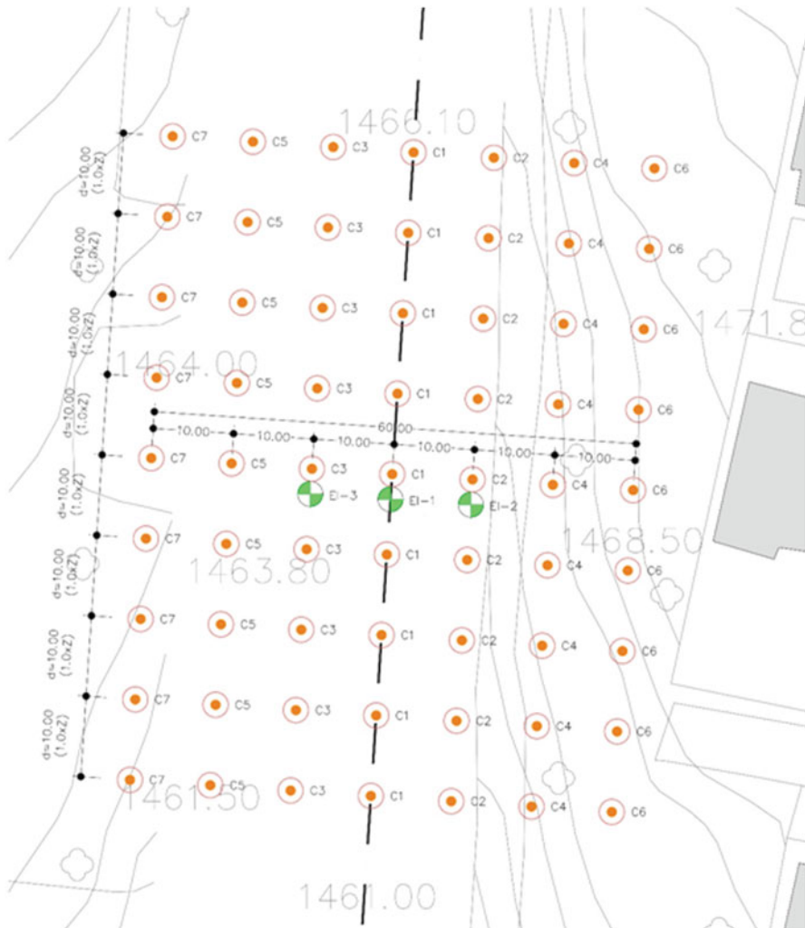
Fig. 8.39 Planimetric layout of benchmarks and strain gauges/clinometers
