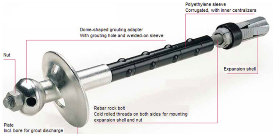
Fig. 6.33 CT-Bolt system components (by DSI, modified). The CT-Bolt system allows the installation of the bolt and its secondary cementation through a PVC sheath that provides an excellent protection against corrosion and guarantees the element durability
