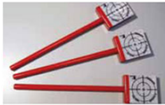
Fig. 8.3 Optical targets: location on the monitored section, installation detail
