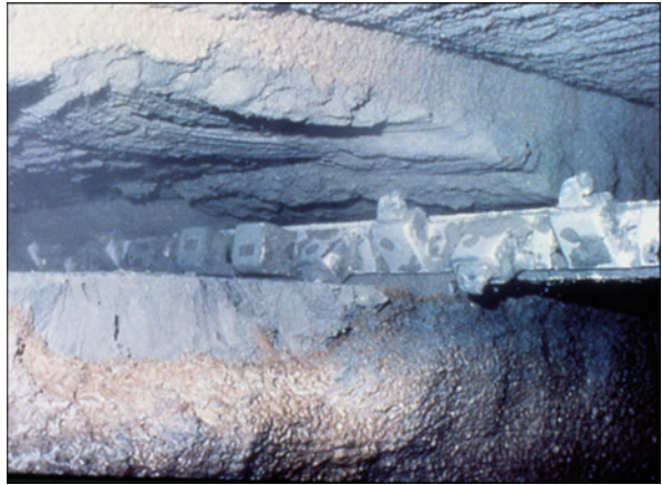
Fig. 6.45 Precutting equipment: Detail of the pronged cutting blade. (By Rodio)
