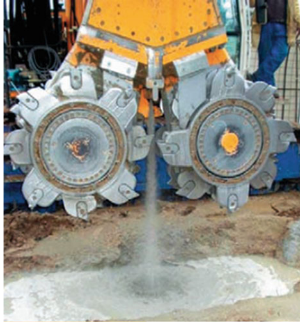
Fig. 6.20 Cutter head used for Cutter Soil Mix. (by Bauer)
