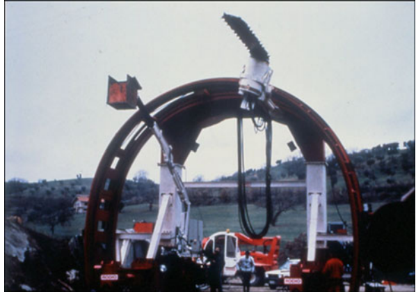
Fig. 6.44 Precutting equipment: The pronged blade is mounted on a structure with the shape of the tunnel to be excavated. (By Rodio)
