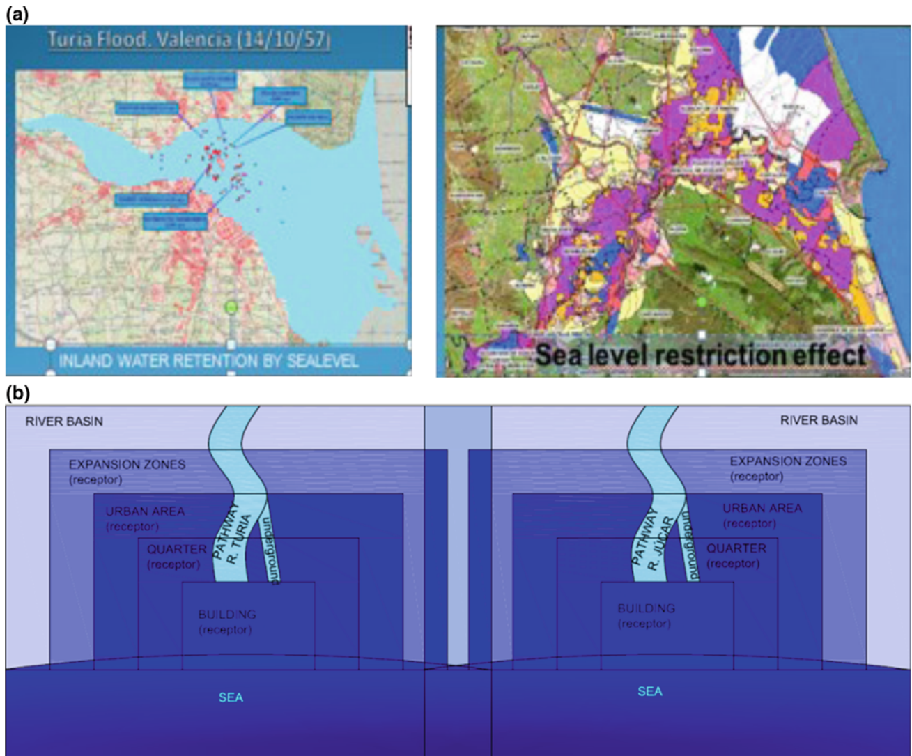
Fig. 29.2 a Flooding effect of the “cold drop” phenomena on Valencia Area: left , on Turia Basin; right , on Jucar basin. b Overlapping of Turia and Jucar floods on Valencia Area
