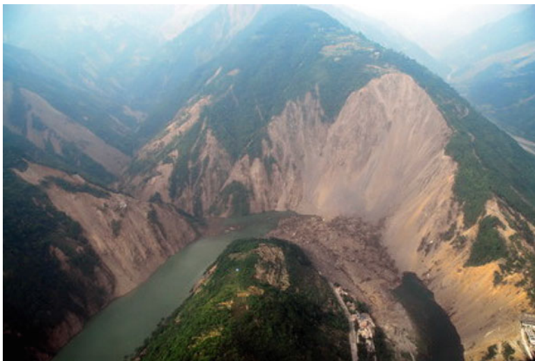
Fig. 1.46 A Quake lake caused by slope failure (2008 Wenchuan earthquake, China) (Institute of Mountain Hazards and Environment, Chinese Academy of Science (CAS), by Xiaogang Zhang)
