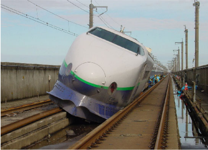
Fig. 1.78 Derailement of Shinkansen due to strong ground motion (2004 Niigata-Chuetsu earthquake)
