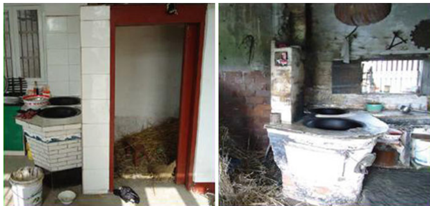
Fig. 3.4 Pictures of two brick stoves tested in this study. The structures of these two stoves were similar with two pots in the middle and an outdoor chimney. These two stoves had different usages. The stove in the left was a new built one (about 1 year ago), and the right one was an old stove used for about 15 years. Reprinted from Environmental Pollution 184, Wei et al., Field measurement on the emissions of PM, OC, EC and PAHs from indoor crop straw burning in rural China, 18–24, with permission from Elsevier
