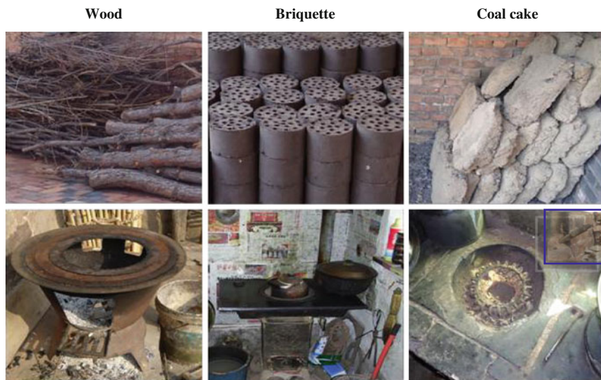
Fig. 3.3 Pictures of three fuel/stove combinations investigated in this study. For left to the right wood, honeycomb briquette, and coal cake burned in a simple metal stove, an improved metallic stove with a chimney and a brick stove with an outdoor flue pipe, respectively. Reprinted from Shen et al. (2013) with permission of American Chemical Society
