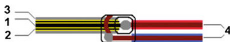
Fig. 5.11 Cutaway view of the integrated working-counter electrode: 1 platinum wire, 2 glass tube, 3 titanium tube, 4 cable. Dimensions are not in scale. Reprinted with permission from Ref. [63]. Copyright 2011 Springer
