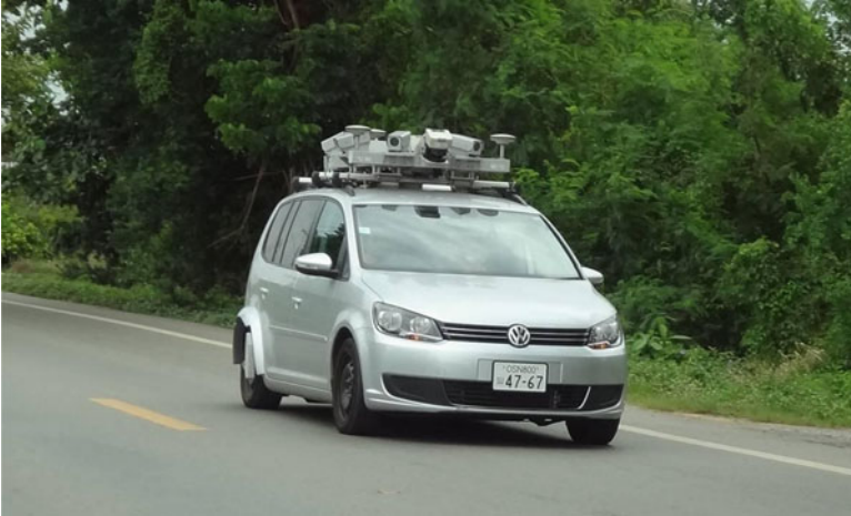
Fig. 7.6 Road inspection vehicle
