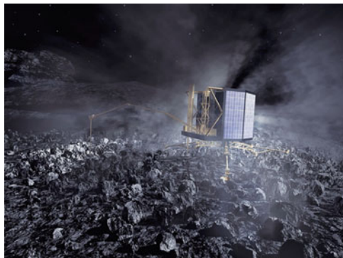
Fig. 9 This artist's impression shows the ROSETTA lander Philae anchored to the comet's surface, where it will work for a minimum mission target of 65 h, although its operations may continue for many months. The lander structure contains the COSAC experiment, a multicolumn GC-TOFMS. Chiral stationary phases will afford the separation of enantiomers detected in the cometary ice. The lander also carries a drilling system to collect samples of subsurface material for analysis. Reproduction with permission of ESA/AOES Medialab
