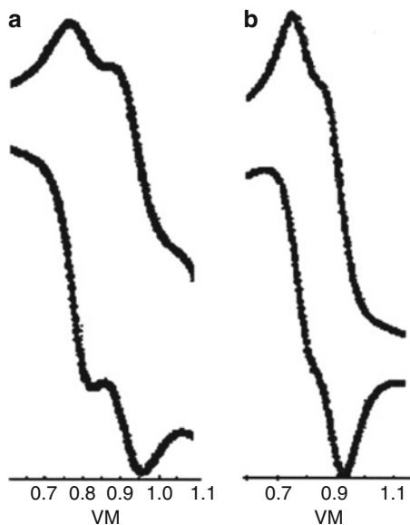
Fig. 10 CVs of (a) a 2.0 mM 9 solution in 0.10 M \text{Bu}_4\text{NPF}_6/\text{MeCN} ; (b) 9 + four times excess of \text{Zn}^{2+} . Potential scan rate of 100 mV/s
