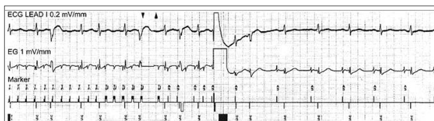
Fig. 2. Intracardiac electrogram and a marker channel showing the detection and shock termination of an episode of atrial tachycardia in a Jewel AF dual-chamber defibrillator. TF interval below atrial tachycardia detection interval, TD atrial tachycardia detection, AS atrial sensed event, VS ventricular sensed event
