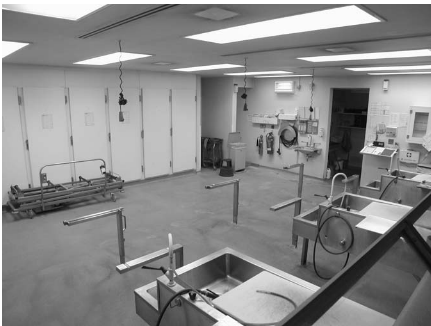
FIGURE 1.4. Mortuary with access to refrigerators from one side. (Courtesy of Mr. Dean Jansen, Whittington Hospital.)
