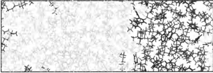
Fig. 4. Dynamic state of the PchMA-co-PGMA-polymer and solvent at a simulation time of 2.0 ns (light gray: polymer, medium gray: n-heptane, black: benzene).
