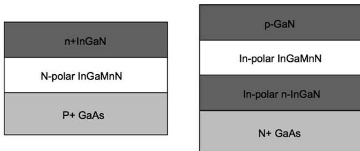
**Fig. 12.7** Proposed InGaN IBSC structures. For N-polar samples, due to the influence of electric fields, the structure shown in (a) should be appropriate. For In(Ga) polar samples, the structure shown in (b) is more appropriate
