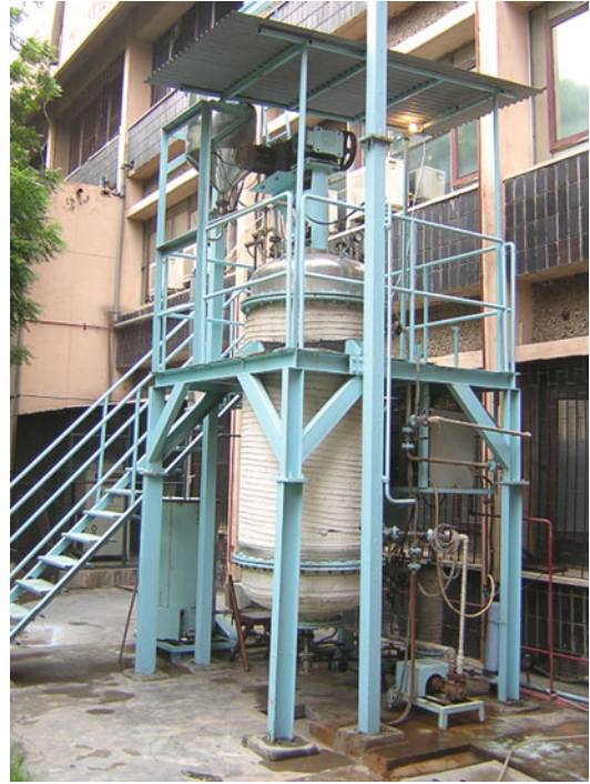
Fig. 2.1 1,200 L packed bed bioreactor. The reactor is a stand-alone unit and operates in all weather conditions
