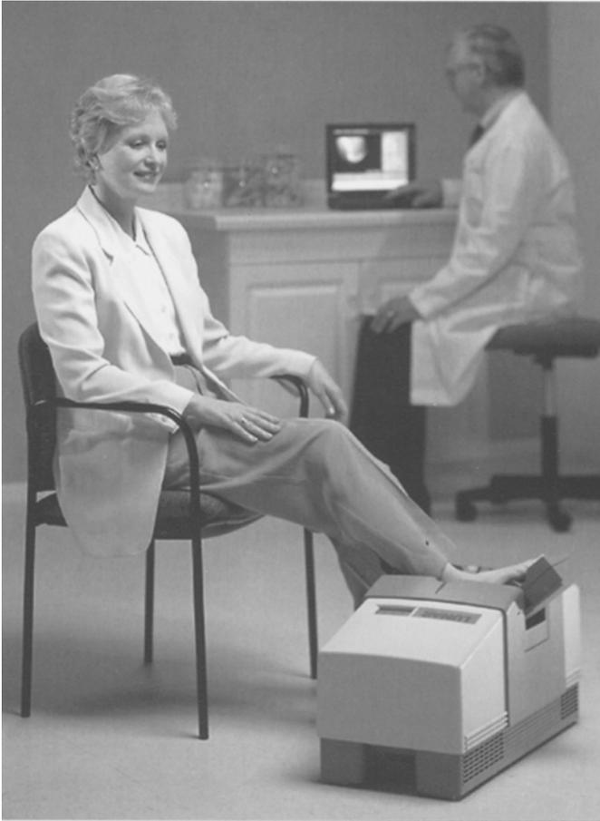
**Fig. 4-23.** GE Lunar PIXI®. A peripheral dual-energy X-ray absorptiometer shown here in the configuration used to measure bone density in the calcaneus. The device can be reconfigured and used to measure bone density in the forearm. (Photograph courtesy of GE Healthcare, Madison, WI.)
