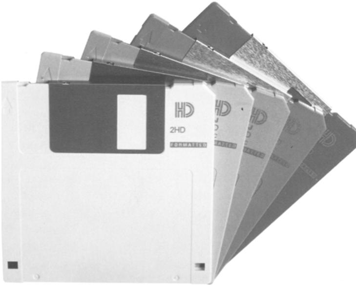
**Fig. 5-13.** Standard 1.44 MB, 3½-in. floppy disks. The designation HD can be seen in the upper right-hand corner. The read-write protect tab is seen on the lower left and is accessible from the back of the disk. (Photograph<sup>®</sup> Hemera Technologies, Inc.)
