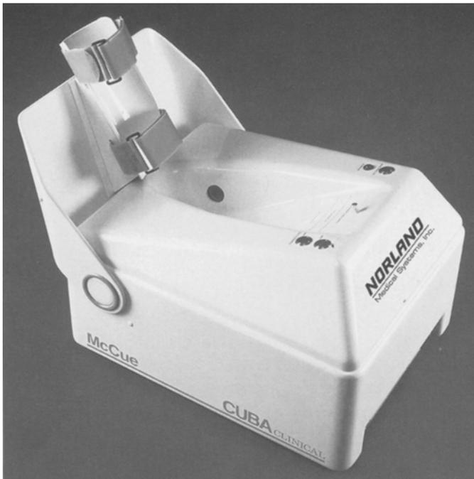
**Fig. 4-32.** McCue C.U.B.A. Clinical™. A peripheral quantitative ultrasound device used to measure the calcaneus. (Photograph courtesy of CooperSurgical Norland, Trumbull, CT.)
