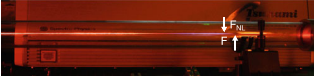
Fig. 1.1 A femtosecond filament obtained by loosely focusing pulsed femtosecond laser radiation into an argon filled gas cell. Initial pulse energy and duration are about 1 mJ and 45 fs, respectively. F and F_{NL} denote linear and nonlinear focus, respectively
