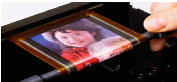
Fig. 10.2 Photograph of a flexible AMOLED display, driven by OTFTs, rolled around a 4 mm radius cylinder. (Reprinted from [4] with permission of SID)
