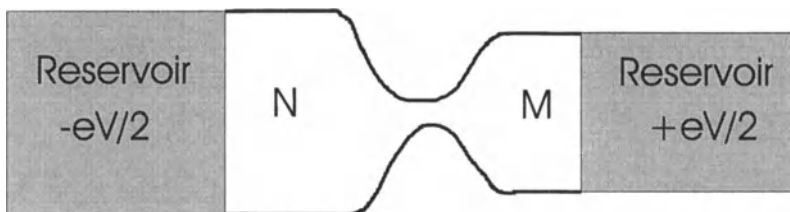
Fig. 6.1. Schematic representation of a ballistic point contact. The reservoirs on the left and right fully absorb the incoming electron waves. The lead on the left has a width, which admits N conductance channels, and the one on the right has M channels
