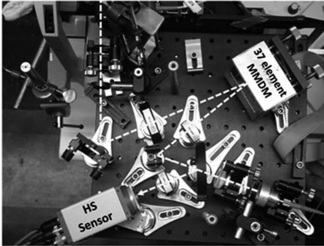
Fig. 10.5 Experimental AO setup attached to a commercial OCT instrument (OCT 1 Carl Zeiss Meditec AG, Dublin, California) used for high-resolution imaging of the living retina in 2003. The system was developed at the University of Vienna, Austria, in collaboration with the University of Murcia, Spain
