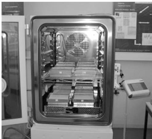
**Fig. 2.6** Cups inside a climatic chamber
