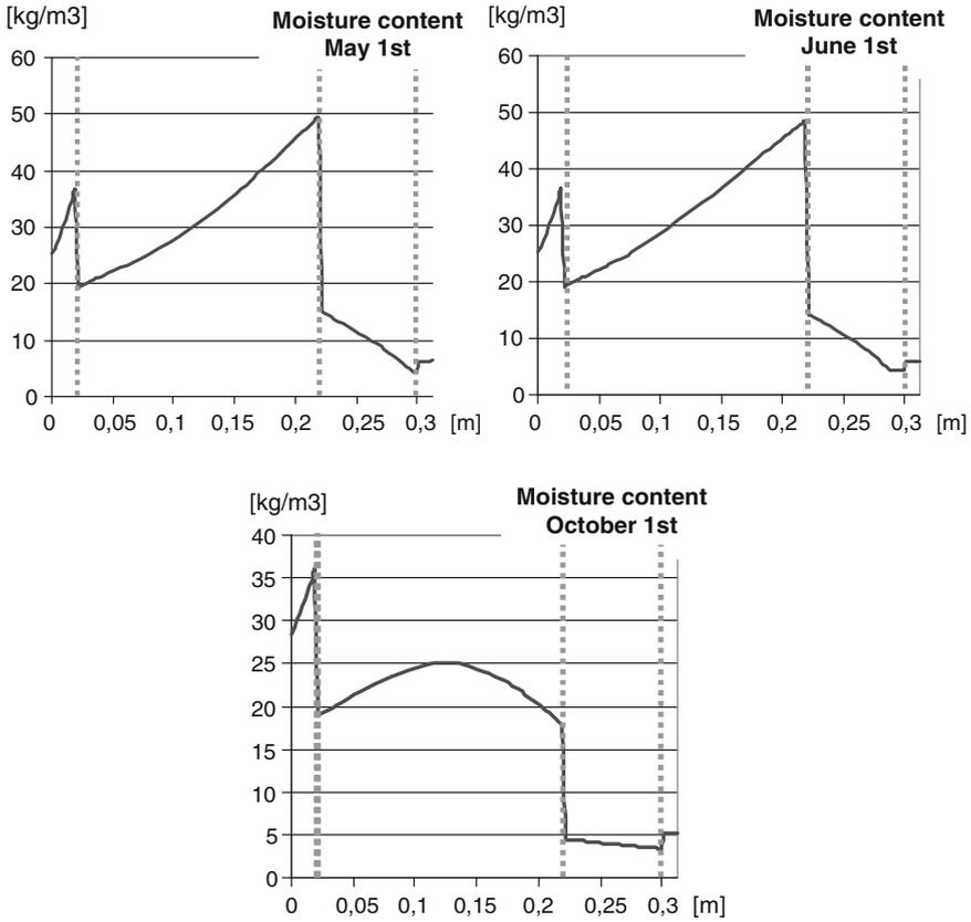
Fig. 4.4 Component moisture content profiles
