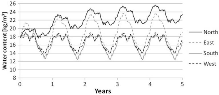
**Fig. 4.6** Variation of water content on solid brick masonry with orientation (maximum WDR load)
