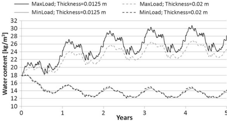
**Fig. 4.11** Variation of water content on solid brick masonry for different mineral plaster thickness and WDR loads, for the North direction
