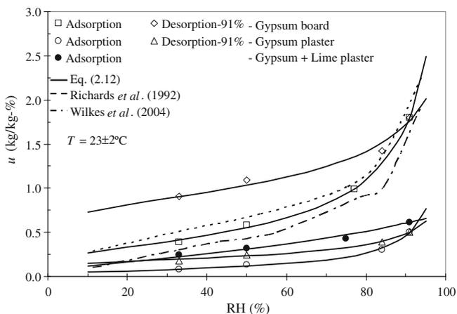
**Fig. 2.10** Sorption isotherms for three types of plaster tested and comparison with other results, presented in literature, for the case of gypsum board
