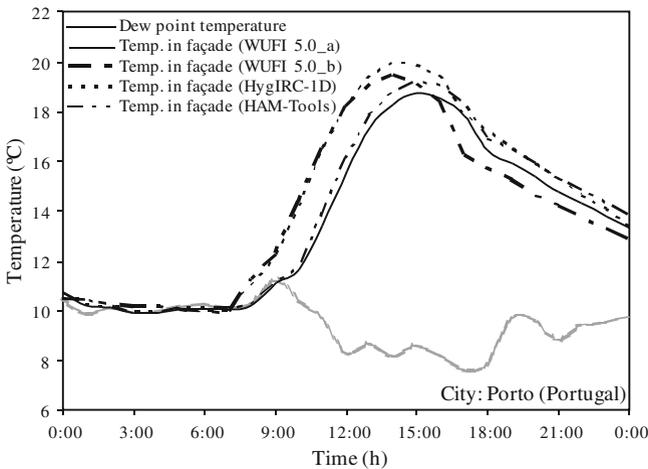
**Fig. 4.15** Surface temperatures obtained by each hygrothermal model for Porto (23-January)
