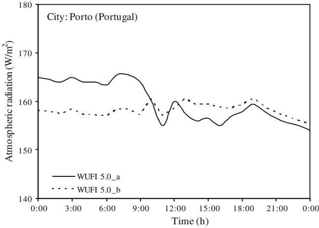
Fig. 4.17 Atmospheric radiation in a vertical plane in Porto (23-January)
