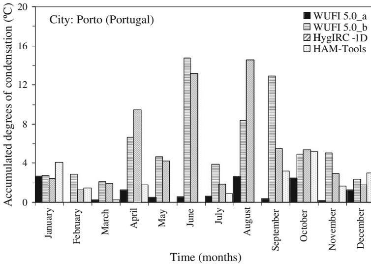
Fig. 4.18 Sum of positive differences between  $T_{dp}$  and  $T_{surf}$  for Porto
