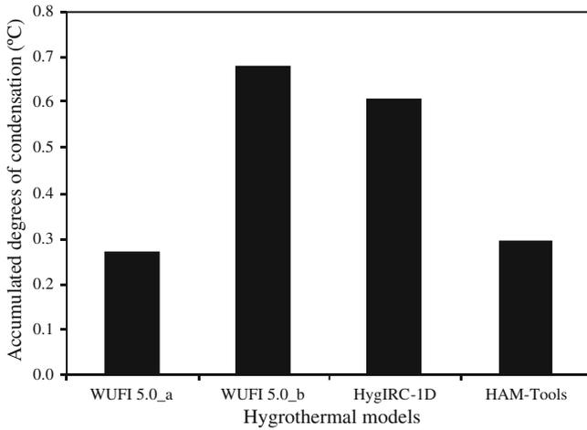
**Fig. 4.16** Sum of positive differences between  $T_{dp}$  and  $T_{surf}$  for Porto (23-January)
