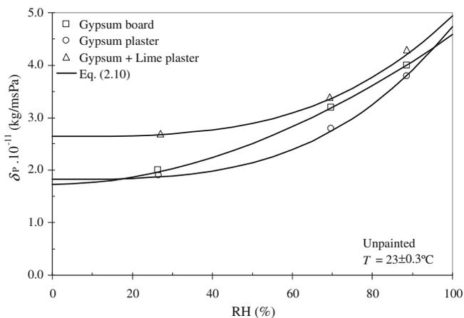
**Fig. 2.7** Water vapour permeability for different specimens tested, at 23 °C, and curve fit
