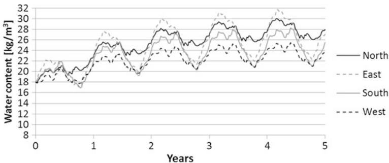
**Fig. 4.12** Variation of water content on solid brick masonry with exterior mineral plaster with  $\alpha_s = 0.2$
