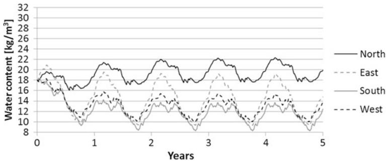
**Fig. 4.13** Variation of water content on solid brick masonry with exterior mineral plaster with  $\alpha_s = 0.6$
