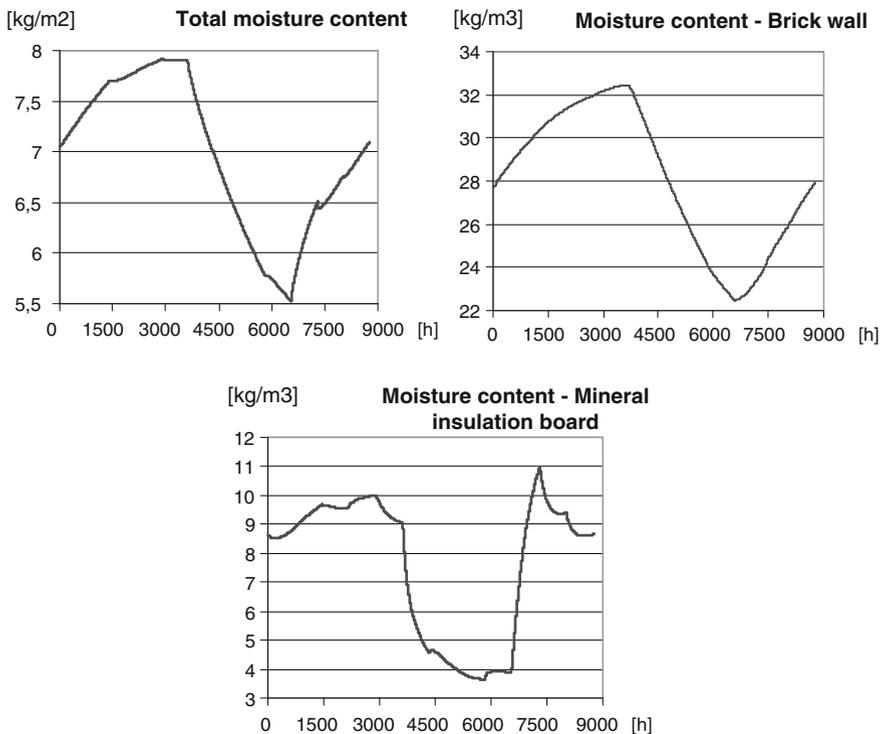
Fig. 4.3 Component moisture content variation over time
