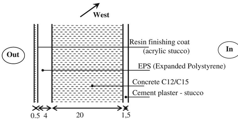
Fig. 4.14 Wall construction details (dimensions in cm)
