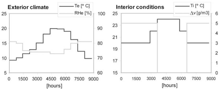
**Fig. 4.2** Boundary condition for simulation
