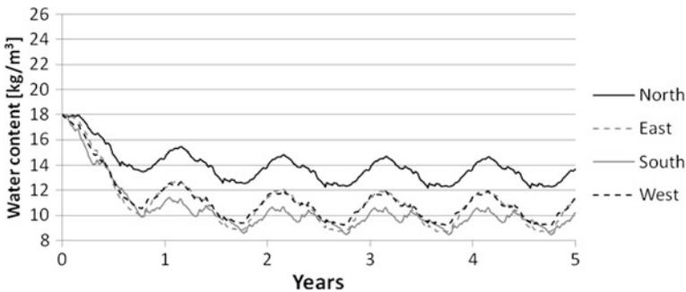
**Fig. 4.10** Variation of water content on solid brick masonry with orientation (minimum WDR load)
