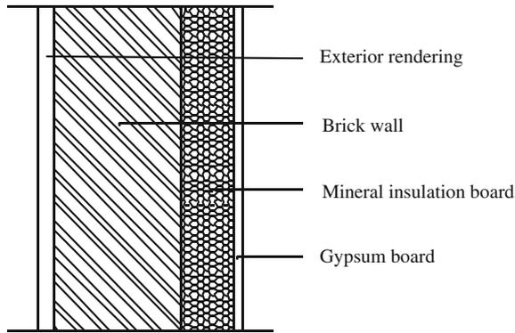
**Fig. 4.1** Building component under study—exterior wall with interior insulation
