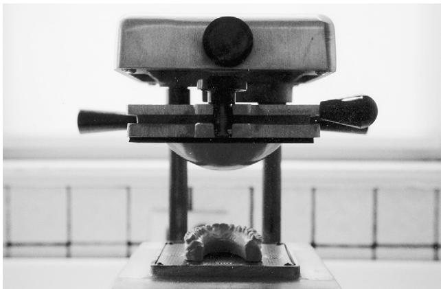
FIGURE 14-30. Ethylene vinyl acetate heated and beginning to droop while model sits ready on vacuum platform. (Courtesy of SportsDDS.com, Hollis Park Gardens, NY.)
