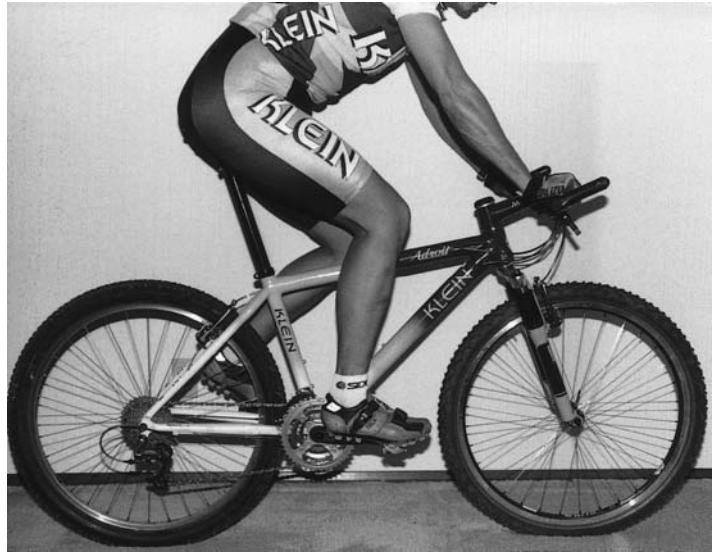
Fig. 36.2 Saddle fore–aft positioning: with the cranks parallel to the floor the ‘average’ rider will find that a good starting position is with the tibial tuberosity over the pedal spindle.
