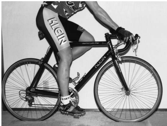
Fig. 36.3 Seat height: at the bottom of the pedal stroke the knee should have a slight flexion angle.
