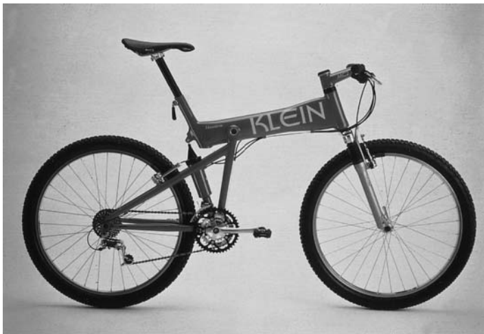
Fig. 36.1 Although the traditional double-diamond frame configuration is still most prevalent, alternative geometries are becoming more common.
