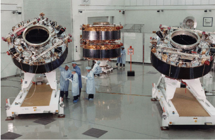
Fig. 3.1 Assembly of four Cluster spacecraft. Courtesy of European Space Agency
