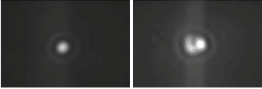
Fig. 3.16 Left: A single optically trapped 3.0\ \mu\text{m} diameter bead; Right: multiple (2 or maybe 3) optically trapped 3.0\ \mu\text{m} beads. The air pressure is 752 torr. The powers of the two counter-propagating beams are 119 and 100 mW
