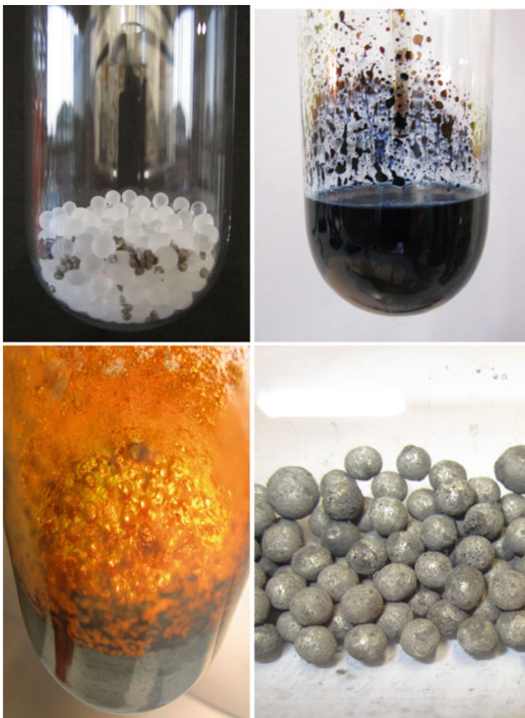
Fig. 1 Activation of commercially available calcium with liquid ammonia; Top left : Calcium granules and glass balls are placed in the Schlenk flask. Top right : Dissolution of calcium in liquid ammonia leads to a dark blue solution. Bottom left : During removal of ammonia calcium bronze forms. Bottom right : Activated and pyrophoric calcium powder is deposited on the surface of the glass balls after removal of all ammonia
