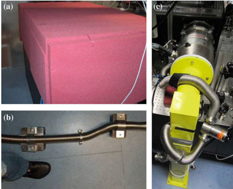
Fig. 4.4 a Protection housing of the laser against mechanical vibrations and air fluctuations. b Vibration-damping heavy iron blocks attached to the bellows connecting the pre-vacuum pump with the turbo pump. c Mounting of the turbo pump and connection to the vacuum chamber containing the enhancement cavity (see text for details)
