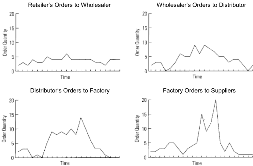
Fig. 2. The Bullwhip Effect or Increasing Variability and Size of Orders Up the Diaper Supply Chain
